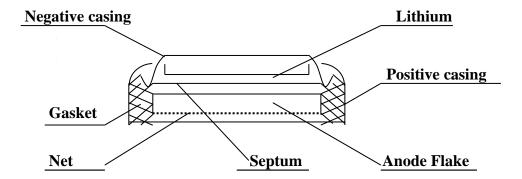
Chemical System: The coin type lithium manganese dioxide battery uses lithium as the negative active material, MnO2 as the positive active material, and an organic electrolyte solution.
